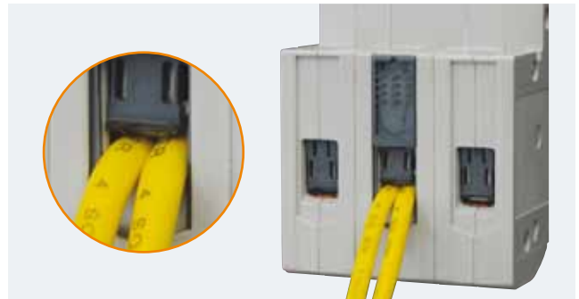
Terminals can accommodate 2 wires of same cross section (Solid up to 2 X 10 mm 2 and finely stranded with end sleeve up to 2 X 4 mm 2 ) without twisting wire strands facilitates easier and safe wiring
